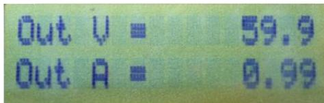
Output Screen shows the voltage on and current through the Pump Motor terminals.
